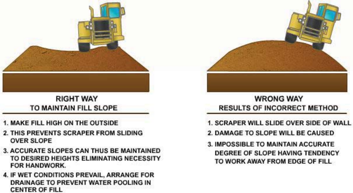
Figure 18-21 – Proper placement to fill material.
