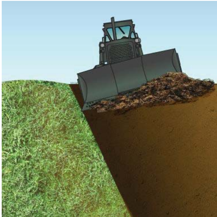
Figure 19-27 – Angle blade ditch cut.
